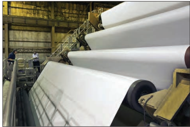
Figure 15 Inclined calender at Resolute Forest Products printing paper machine at Catawba, USA. Image: www.resolutefp.com .
