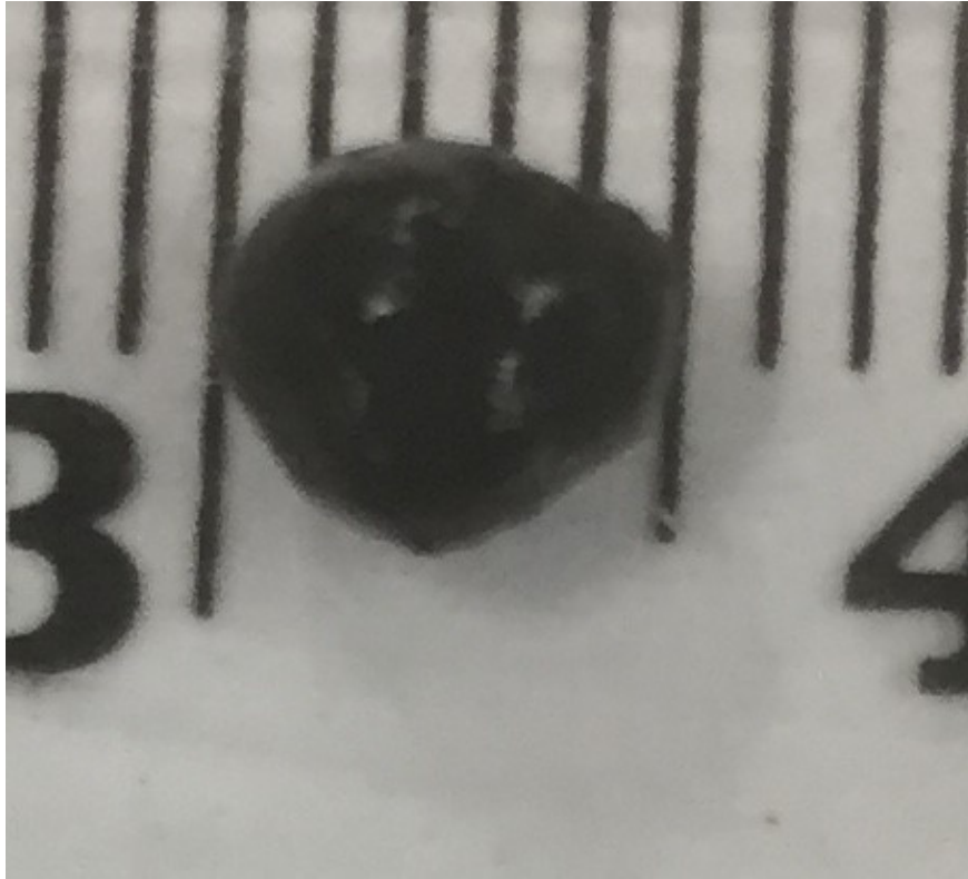
Figure 5 Size, shape, and color of biomass granules after the first week of recommissioning.
