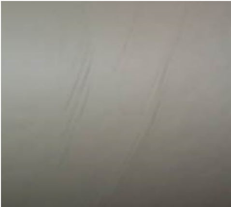
Figure 13. Wrinkle problem on parent roll surface.
