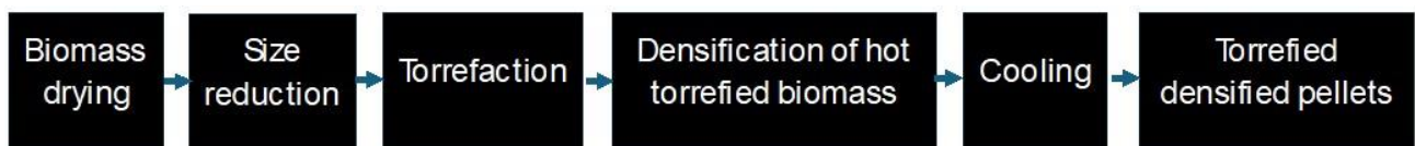
Figure 12: Torrefaction and densification process
