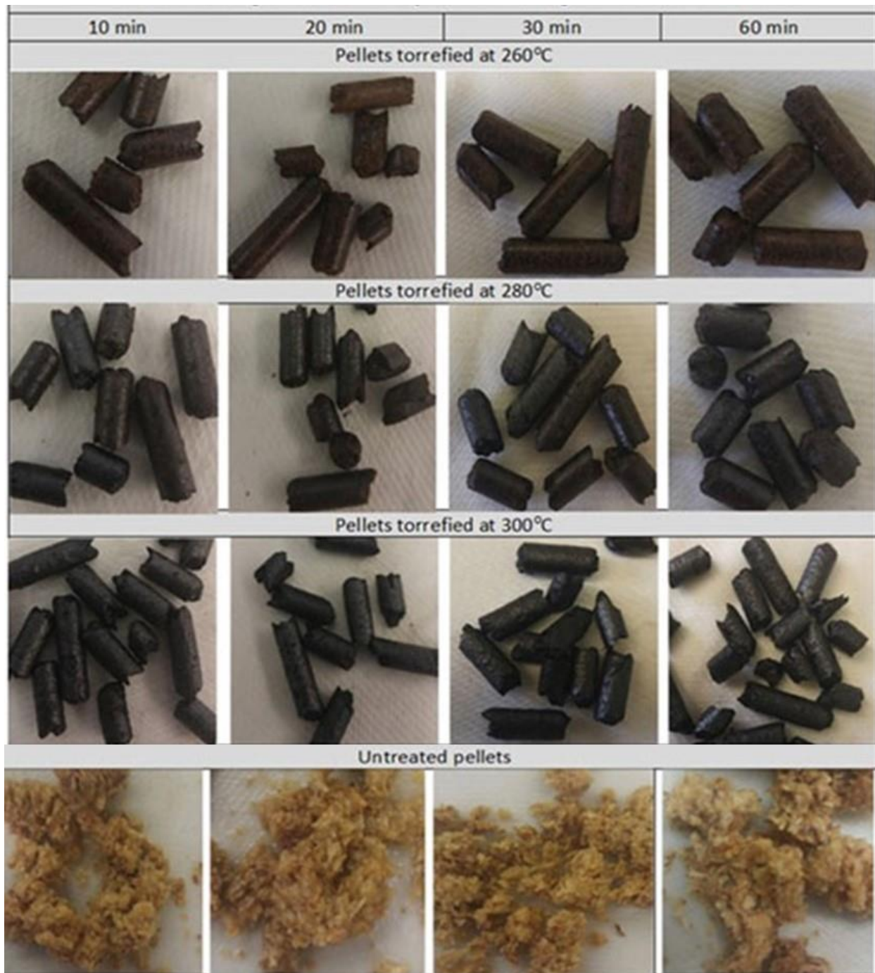
Figure 13: Behaviour of raw and torrefied pellets immersed in water.
